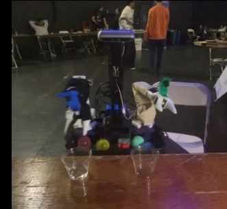
Calhacks 2025: Integrated SmoIVLA to map human gestures to robot actuation commands.
