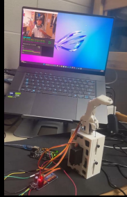
Finger Test Bed: Validated Nitinol wire flexible properties for tendon driven approach. Mediapipe for joint angle detection.
