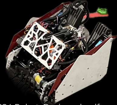
2024 Robot: Designed, self fabricated and built the drivetrain, lift, intake, outtake subsystems.
